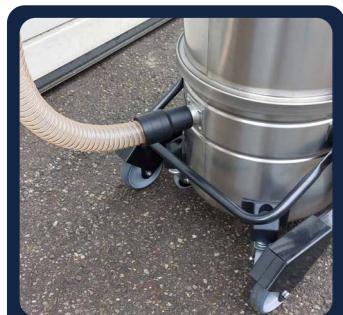
The Ø40 mm spiral PU metal hose is abrasion-resistant and connects directly to the removable tank.
