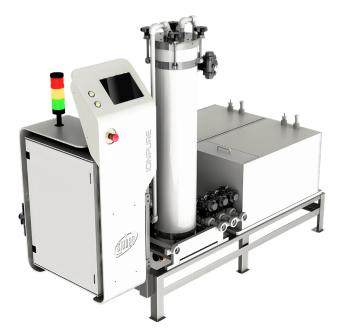
IONPURE<sup>™</sup> continuously eliminates metals polluting the chromium (III) baths in order to guarantee optimal concentration and constant parts quality.
