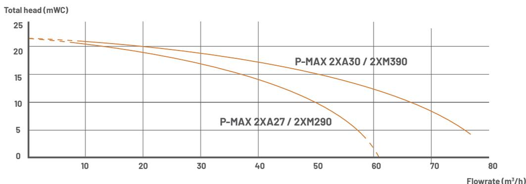
\*Flow rates measured on 8 L-TECH cartridges, with water at 20°C. Variable flow rates depending on filter assembly.
